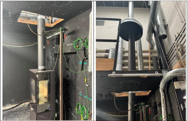
Details, test flue, extraction hood and insulated chimney part
