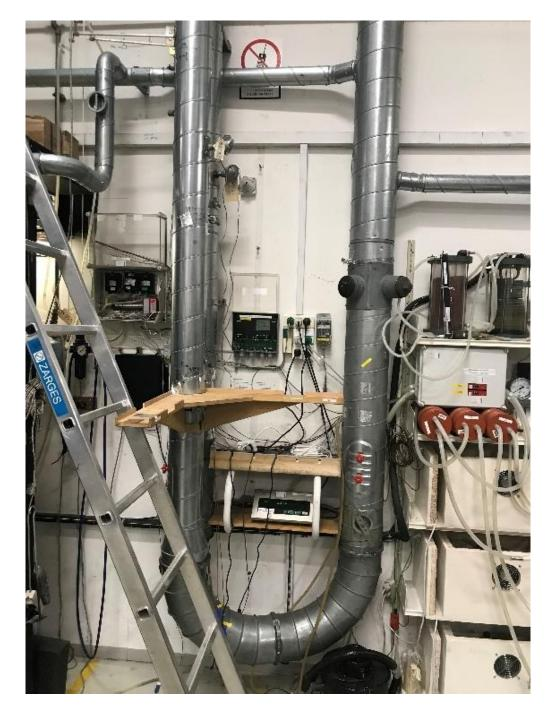
Details, pitot tube, temp sensor, sampling and traverse parts of the FFDT
