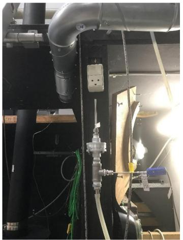
Placement of ambient blank filter holder
